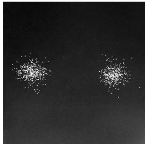
(d) Constellation plot for a wireless transmission of a BPSK data frame (low SNR).
