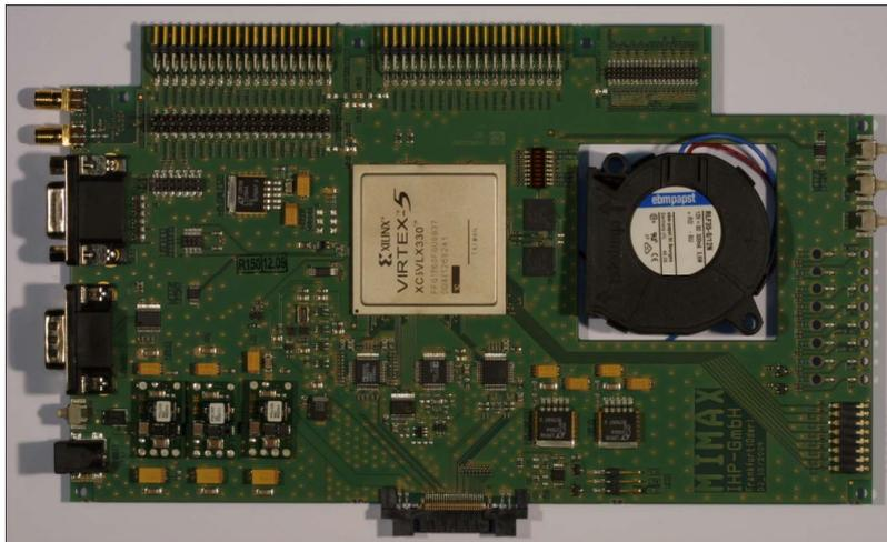
**Figure 8.1:** MIMAX baseband board (135 mm × 225 mm).
