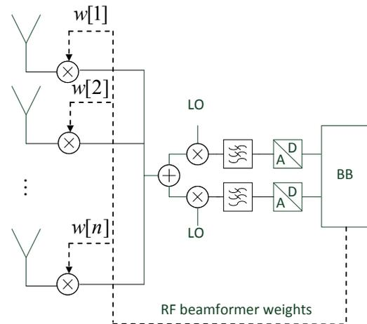
Figure 1: Analog antenna combining in the RF path for MIMO communications systems. Exemplarily shown for a direct-conversion receiver.
