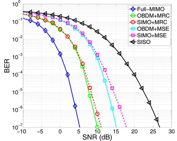
Figure 4: BER performance of the evaluated schemes with time and frequency precoding.
