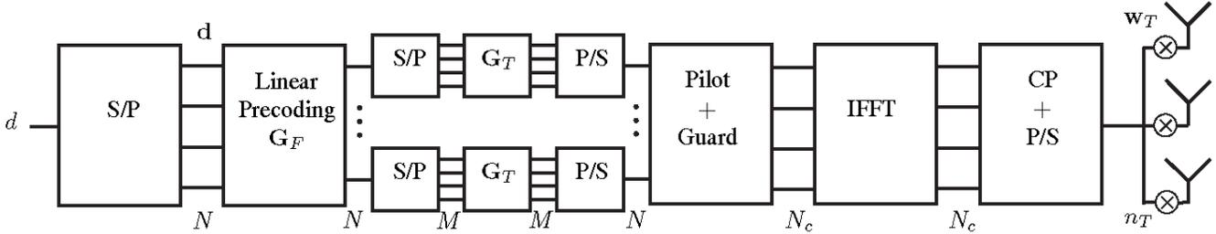
Figure 2: Block diagram of the OFDM-based transmitter with analog antenna combining. The receiver diagram is equivalent.
