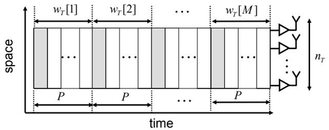
Figure 3: Distribution of a transmission block. The grey columns denote the  $M$  time and frequency precoded OFDM symbols of one block, which are transmitted using  $M$  different beamformers. In this example the beamformers remain fixed during the transmission of several ( $P$ ) OFDM symbols.
