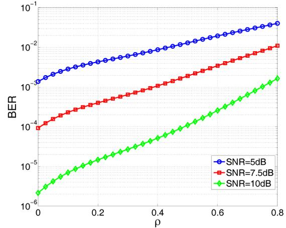
Figure 6: BER of the proposed scheme as a function of the exponential channel parameter.
