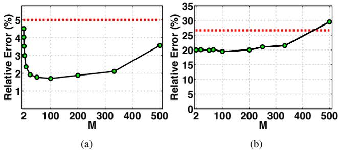
Figure 3. (Ex-in-Sect VIII-A-VIII-B) Relative error (%) obtained with APIS as a function of the number of epochs  $M = \lfloor \frac{T}{T_a} \rfloor$  (solid line) and the particle splitting method [15, pages 495-498] (dashed line), (a) for the example in Section VIII-A and (b) for the example in Section VIII-B.
